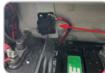
The windlass breaker is located in the bilge access compartment above the batteries
