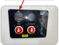
The windlass breaker is located on the battery switch panel located behind the dash in the head/console compartment.
