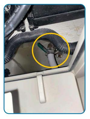
Access to the Marine Head Discharge Seacock is located in the Fwd head area accessed through the battery storage compartment hatch.
