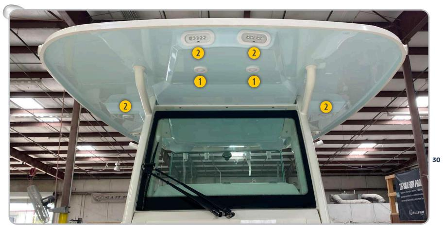
The standard hard top is equipped with courtesy lights, spreader lights, docking lights, an anchor light, two speakers, an overhead electronics panel and PFD Storage Area.
