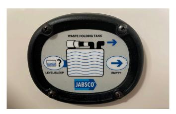
**Jabsco Tank Monitor installed with Overboard Discharge**
