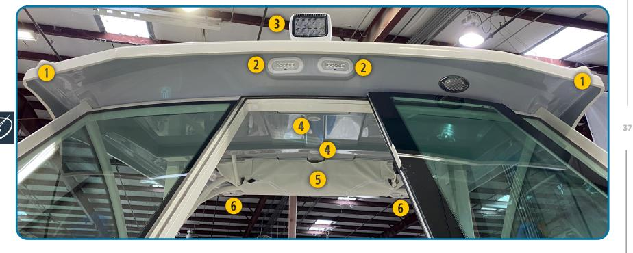
The standard hard top is equipped with navigation lights, courtesy lights, spreader lights, docking lights, an anchor light, two speakers, 6 rocket launchers, and overhead PFD Storage.
