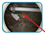
Access to the Marine Head Discharge Seacock is located in the Mid-Ship In-Floor Ski Locker. it is the same access plate used for the Fwd Bilge pump.
