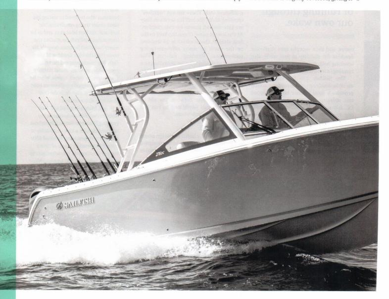
Sailfish spent a lot of time balancing the size and shape of the strakes on the 276 DC to minimize drag underway while still helping to cushion the boat as it runs through a sea state.
