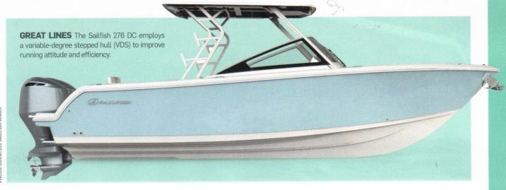
Deadrise"), which Sailfish acquired years ago. Since that time, Sailfish has modified the design to reflect modern technology. This includes widening the hull aft to carry the weight of heavier, more powerful outboards, and adding a flat spot known as a pad.
