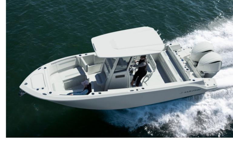
Like all Sailfish boats, the 252 CC features our innovative Variable Degree Stepped (VDS) hull for a smooth, stable ride in any condition. This three hulls-in-one design optimizes performance and stability, with a deep 24-degree step cutting through water, a 23-degree surface reducing friction for efficiency, and a 22-degree outer step enhancing stability at rest.
