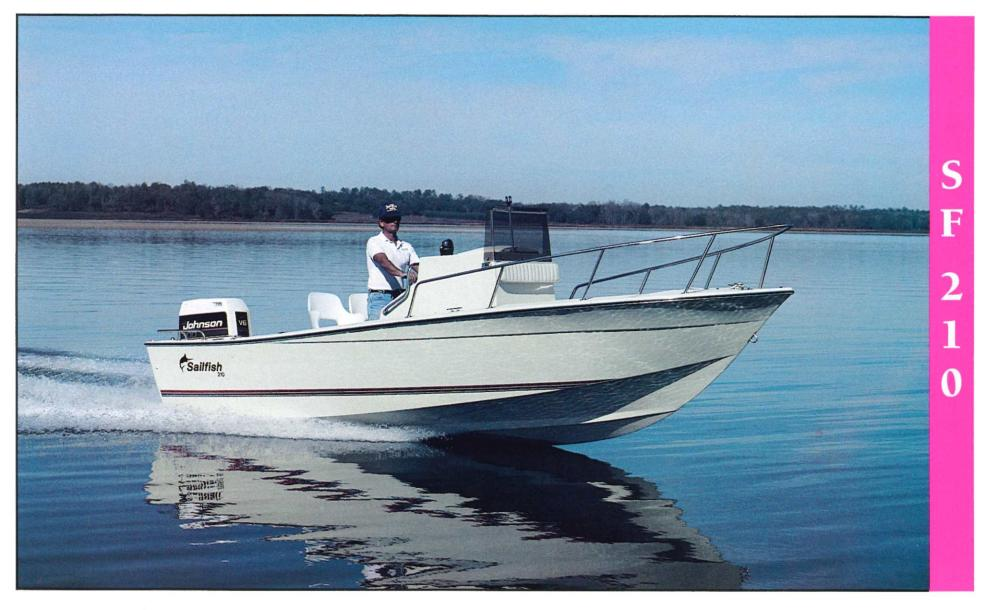
The Sailfish SF 210 offers big center console features in a manageable sized package. Aerated live well, insulated fish box, rope and anchor locker, plus 66 gallon fuel capacity, for long range capability. The large walk in console offers loads of storage, plus a six foot bunk and recessed porta potti area for comfort and convenience. An ideal family fishing boat, the SF 210 is versatile, as well as practical.
