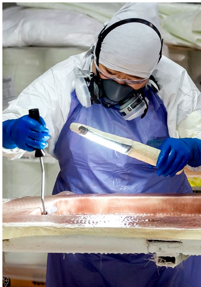
CRAFTED WITH CARE A Sailfish technician applies a coat of fiberglass by hand, carefully rolling each section to eliminate gaps, bubbles or flaws that could compromise its durability.
