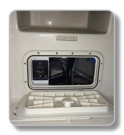
The windlass breaker is located in the bilge hatch below the walk-thru transom door.
