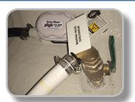
Access to the Marine Head Discharge Sea-cock is located in the Fwd head area, accessed through the Fwd hatch, it is the same access used for the Fwd Bilge pump.
