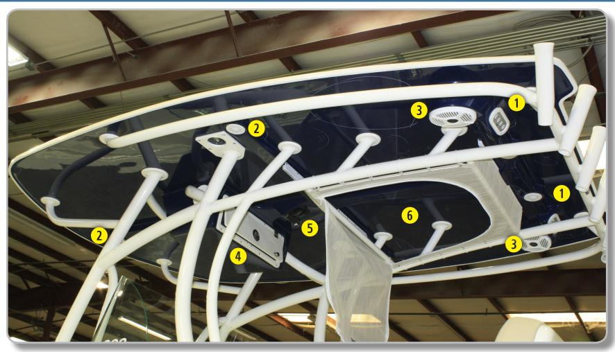
The optional hard top is equipped with courtesy lights, spreader lights, docking lights, an anchor light, two speakers and an overhead storage box.
