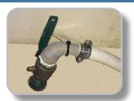
Access to the Marine Head Discharge Sea- cock is located behind the pie plate access in the side of the starboard step to the walk around area.
