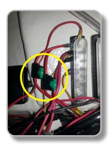
The fuses for both the marine head and the waste tank are located behind the dash in the first panel coming off the bus bar, pictured to the left.
