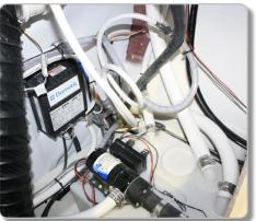
Depending on the equipment in your boat, many of your power options can be accessed by removing the tackle stations in the cockpit. Behind these you will have access to the Air Conditoning, Water Heater and the Fire Boy System, as well as plumbing hoses and wiring.
