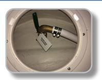
Access to the Marine Head Discharge Sea-cock is located in the Driver's side storage area, accessed through the pie plate in the floor.
