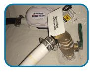
Access to the Marine Head Discharge Seacock is located in the Fwd head area on the floor, it is the same access plate used for the Fwd Bilge pump.
