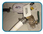
Access to the Marine Head Discharge Seacock (Overboard Discharge is Optional) is located in the Fwd head area on the floor, it is the same access plate used for the Fwd Bilge pump.
