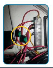
The fuses for both the marine head and the waste tank are located behind the dash in the first panel coming off the bus bar, pictured to the left
