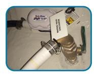
Access to the Marine Head Discharge Seacock is located in the Fwd head area on the floor, it is the same access plate used for the Fwd Bilge pump.
