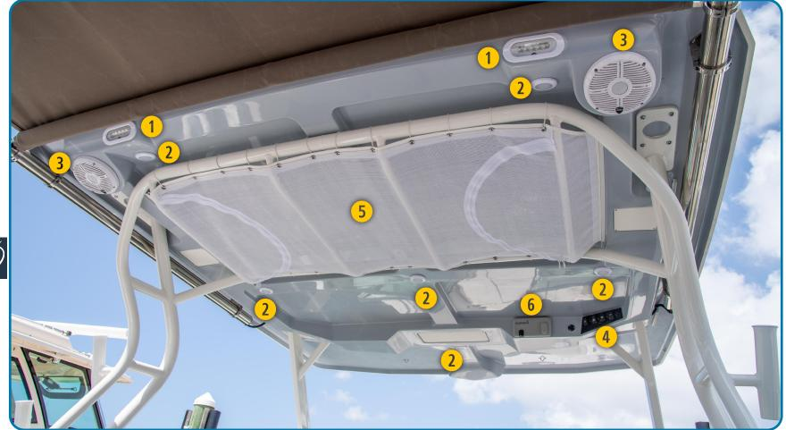
The standard hard top is equipped with courtesy lights, spreader lights, docking lights, an anchor light , two speakers and overhead PFD Storage. Shown with optional SureShade MTF™.
