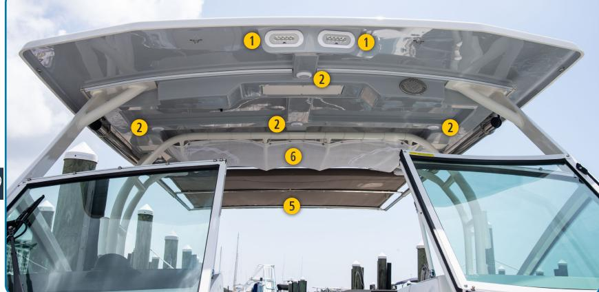
The standard hard top is equipped with courtesy lights, spreader lights, docking lights, an anchor light, two speakers and overhead PFD Storage. Shown with optional SureShade MTF™.
